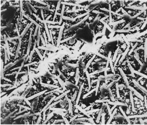
FIGURE 2 Crack deflection by mica crystals in fluorophlogopite glass-ceramics. [After Grossman, D. G. (1977), Vacuum 28 (2), 55–61.]
